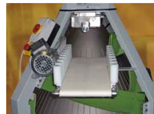
Exit conveyor belt / cinta de salida
